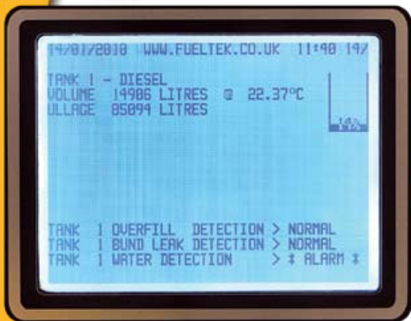
INFORMATION DISPLAYED AT THE FUEL TANK
